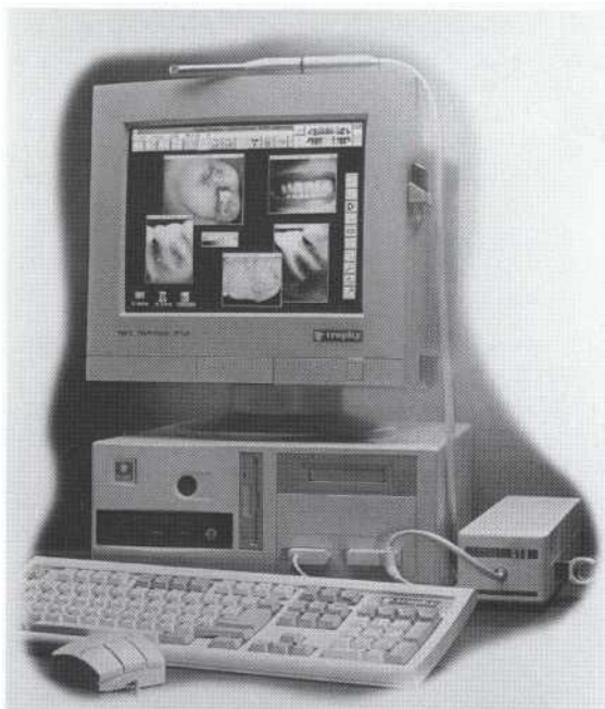
FIGURE 9-31 A digital imaging workstation for the dental operator. The system integrates filmless digital images with an intraoral camera into a standard PC. (Courtesy Trophy USA.)
