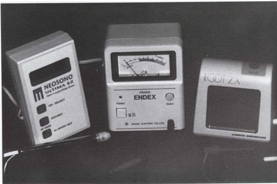
FIGURE 12-30 Examples of impedance-based electronic apex locators. These will function fairly accurately in either a wet or dry canal.
