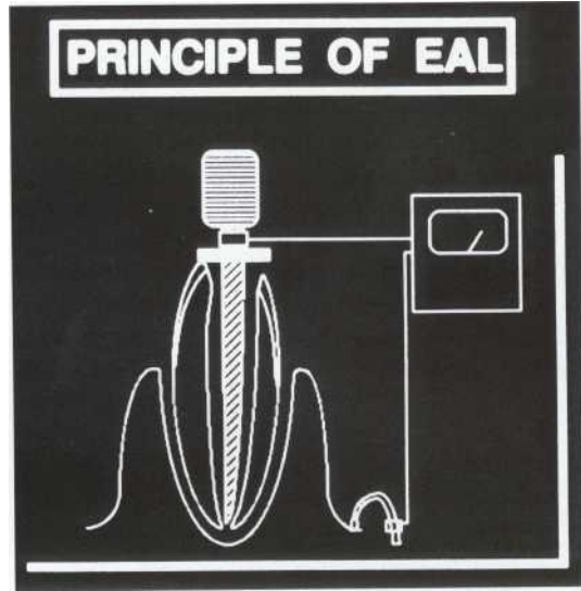
FIGURE 12-29 Electronic apex locators (EALs) operate on direct current, which is supplied by the unit on the upper right. One electrode is in contact with the metal shaft of the file; the other contacts soft tissue, usually by a lip clip. When the tip of the file touches tissue at the apical foramen, current begins to flow.
